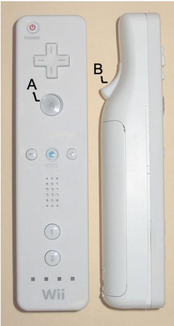
**Figure 1.** The *Wii Remote* (a.k.a. *Wiimote*), the commercial device used to implement *UniGest*. The large A-button is visible on the top of the left *Wiimote*. The B-button is the trigger on the underside, visible on the right *Wiimote*.
