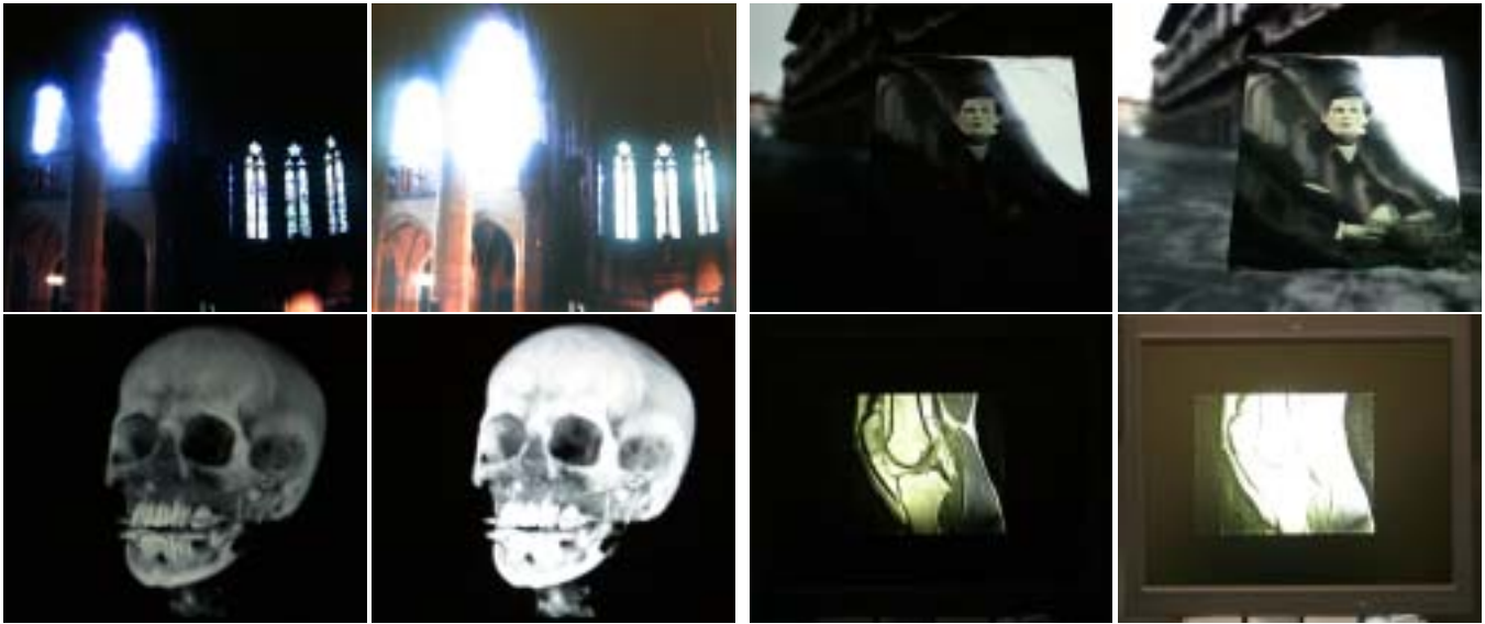
Figure 12: Screen photographs of the different applications we implemented. The exposure times of the two images in each pair differ by 4 stops. Top left: HDR image viewer. Top right: interactive rendering of measured BRDFs. Bottom left: volume rendering. Bottom right: medical image viewer.
