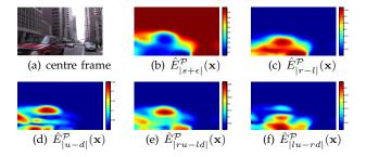
Fig. 4: Distribution of Dynamic Pooling Energies of a Street Sequence from the YUPENN Dataset. (b)-(f) show the decomposition of the sequence into a distribution of pooling energies indicating stationarity/homogeneity in (b) and coarse coherent motion for several directions in (c)-(f). Hotter colors (*e.g.*, red) correspond to larger filter responses.
