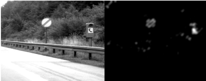
Fig. 3. Left – input image, Right – saliency map. This model reproduces the results presented by Itti et al. (Figure 3 in [6]). The model identifies the phone pole as the most salient area of the image, followed by the traffic sign. See Fig. 1 for details and a view of the whole network.
