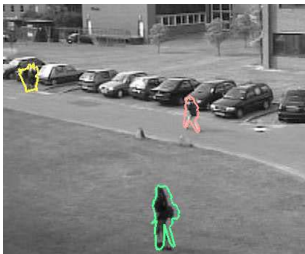
Figure 6. The outline \rho_{1..n} shown as connected points. Distinct objects are marked with different colours.
