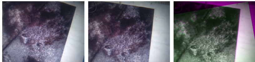
Figure: Left: S_j ; middle: loop closing image I_c . On the right: the transformation of the image registration applied to S_j . The purple color indicates the error of the transformation.
