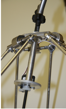
Figure 5: The axial servo is mounted on a platform attached to the center of the gimbal plate.
