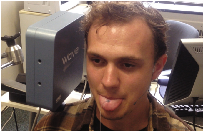
Fig. 2. The wave system and one of its sensors attached to a person's tongue
