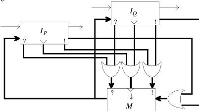
Each disjunction is really many disjunctions, one for each bit in its operands.
