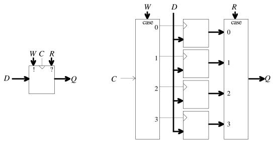
Adding an arrow in the diagram indicates that the flip-flops are edge-triggered.
