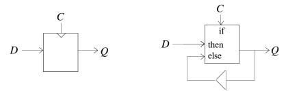
For the circuit to operate correctly, the delay must be small enough that no change to D occurs during the delay preceding the fall of the clock. For the circuit to be as fast as possible, the delay must be as small as possible. There will be a constraint on the minimum delay for electrical reasons, which we do not consider here. With no delay, this circuit is logically equivalent to a standard textbook flip-flop.
