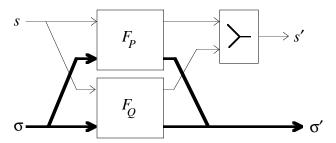
The entire input can go to both programs, but each program produces only part of the output. These outputs together form the entire output.
