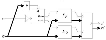
The data output could, alternatively, be selected using the b output without memory. The **if** circuit is easily generalized to a **case** circuit.
