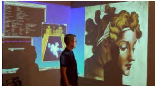
**Figure 1:** Front projection displays suffer from shadowing artifacts when users occlude projector frustums. This is particularly a problem for projector-based immersive environments that involve large numbers of projectors and encourage users to move within the display environment.
