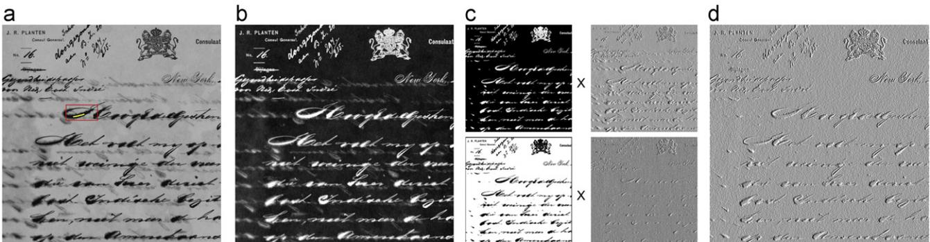
Fig. 3. Gradient map construction for text documents: (a) input image and an user mark-up, (b) similarity map  $S$ , (c) gradients for foreground  $\nabla I_i$  and background  $\nabla I_\lambda$ , (d) gradient composite  $G$ .
