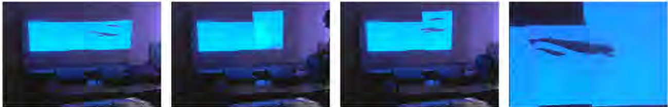
Figure 1: A PC-cluster tiled display using three casually positioned projectors running an unmodified OpenGL application ( Atlantis ). The display geometry is changed by tilting one of the projectors on its side. Camera-based geometric registration has the entire display back in seamless operation in less than one minute .
