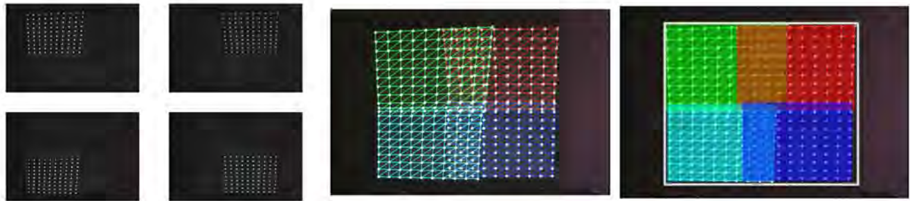
Figure 3: Geometric registration procedure for four projectors. Fiducials from individual projectors are identified in the camera image plane. The fiducials within a given projector form a triangulated mesh. WireGL “tiles” are assigned to each projector.
