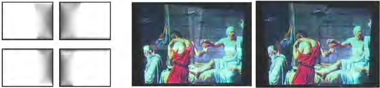
Figure 5: Intensity blending using alphamasks. One mask per projector is generated. This mask attenuates overlapping framebuffers. A 2x2 projector array with and without intensity blending is shown.
