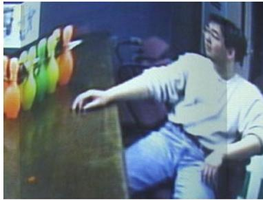
(b) Projected imagery is distorted due to non-planar display surface.
