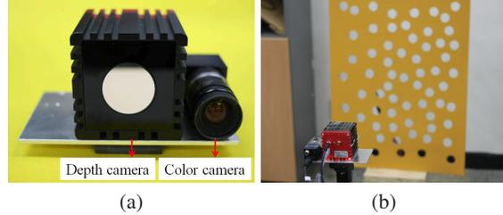
Figure 2. (a) Our imaging setup uses a 3D-ToF camera which captures images at  $176 \times 144$  resolution that is synchronized with a  $1280 \times 960$  resolution RGB camera. (b) Our calibration configuration that uses a planar calibration pattern with holes to allow the 3D-ToF camera to be calibrated.
