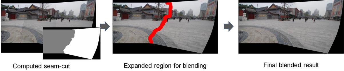
Figure 4. This example shows our blending procedure where a seam-cut is first computed, followed by blending about the seam.
