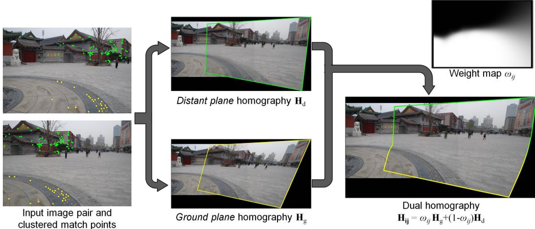
Figure 2. Work flow of our dual-homography computation. Candidate points are first clustered into groups from which two homographies are estimated using RANSAC. A per-pixel weight map  $\omega_{ij}$  is computed to control the blending of the two homographies.
