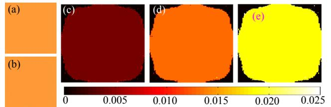
Fig. 10. Difference between the color channels of the object and image planes. (a) object plane, (b) image plane, (c) difference in red channel, (d) difference in green channel, (e) difference in blue channel.
