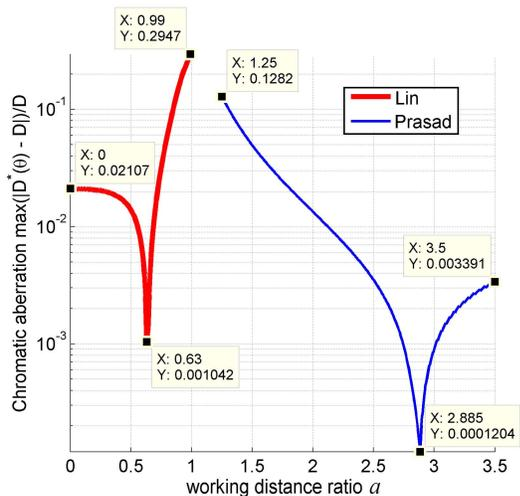
Fig. 5. The chromatic aberration of [3]’s macro-filter and the proposed (Prasad) macro-lens-filter design as a function of the working distance ratio.
