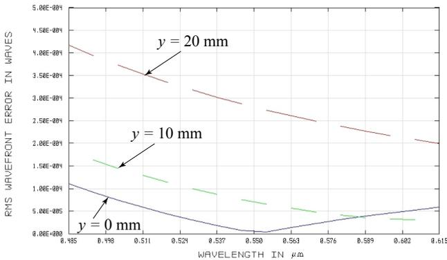
Fig. 7. RMS errors are plotted as a function of wavelength. Blue, green, and red lines indicate rays from three field points corresponding to  $y = 0\text{mm}$ ,  $y = 10\text{mm}$ ,  $y = 20\text{mm}$ .
