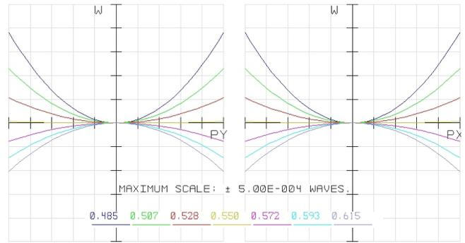
Fig. 9. Optical path differences are plotted as a function of pupil angle and for various wavelength (unit  $\mu\text{m}$ ) samples in the visible range.
