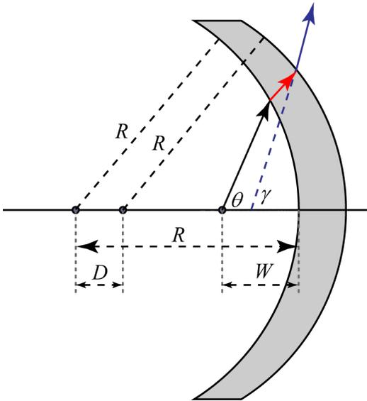
Fig. 1. Illustration of the macro-filter design proposed in [3]. Here, approximate path travelled by the rays  $D \ll R$ , working distance  $W < R$ ,  $R$  is the radius of the two spherical surfaces, and  $n$  is the filter material.
