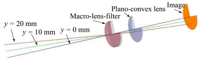
Fig. 6. Illustration of the simulation setup used for Zemax simulation. The front element is the macro-lens-filter, the back element is the plano-convex lens used for focusing the rays from the macro-lens-filter. Red, green, and blue lines indicate rays from three field points corresponding to  $y = 0\text{mm}$ ,  $y = 10\text{mm}$ ,  $y = 20\text{mm}$ .
