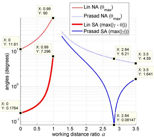
Fig. 4. The numerical aperture (NA) and spherical aberration (SA) of [3]’s macro-filter and the proposed (Prasad) macro-lens-filter design as a function of the working distance ratio.
