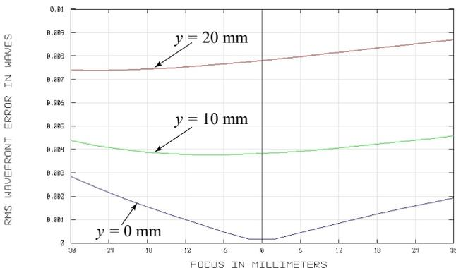
Fig. 8. RMS errors are plotted as a function of longitudinal deviation from the focal point. Blue, green, and red lines indicate rays from three field points corresponding to  $y = 0\text{mm}$ ,  $y = 10\text{mm}$ ,  $y = 20\text{mm}$ .
