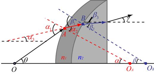
Fig. 3. Detailed illustration of the proposed macro-lens-filter. The definition of all the angles involved in analysis of the macro-lens-filter design are shown here.
