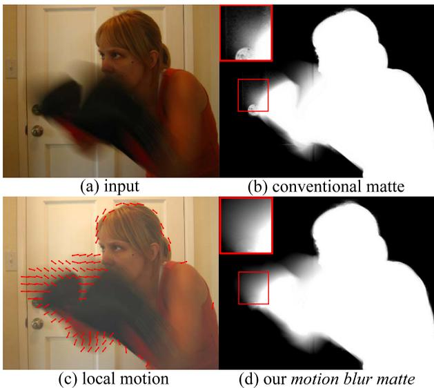
Fig. 1. (a) An image with motion blurred foreground object, (b) conventional matte obtained from closed-form matting [2], (c) estimated local motion, and (d) motion matting using [2] with motion regularization incorporated.
