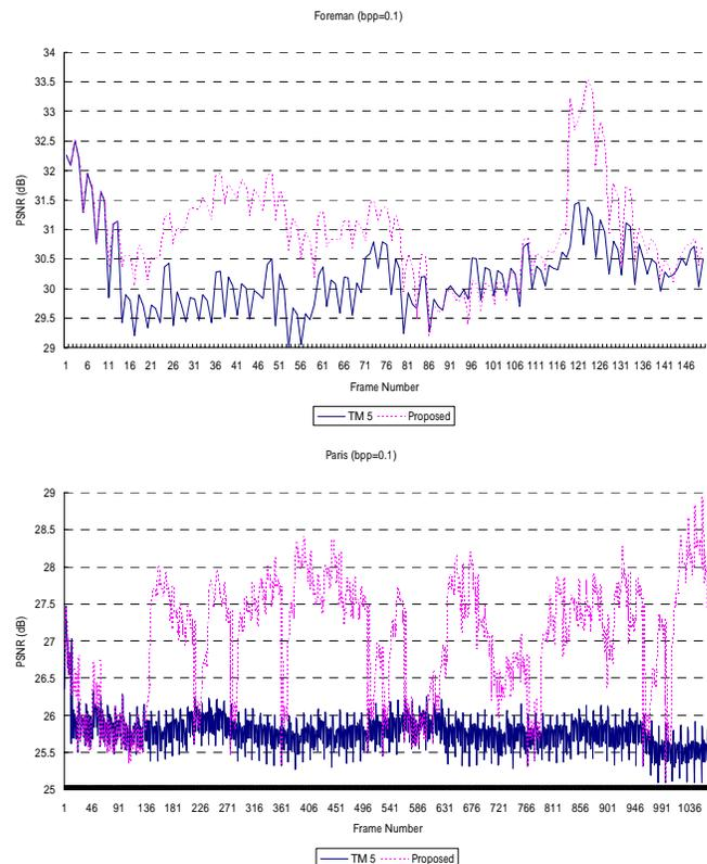
Figure 3: Comparison between TM5 and TM5 with LRU method based on the PSNR value of Y component of each frame for the Paris and Foreman sequencee. (bitrate = 0.1bpp, workingset size = 2, threshold = 10.)
