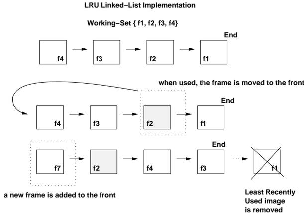
Figure 2: LRU frame replacement: A list is kept of all of the frames. When a new frame is added, or a frame in the working-set is chosen to replace a candidate I-frame, it is moved to the front of the list. The least recently used frame is always the at end of the list.
