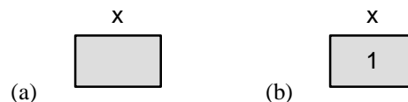
Figure 2. (a) A variable x is declared, but not initialized (b) a variable x is initialized with the value 1.
