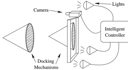
(b) An intelligent controller can manipulate lighting intensities and camera intrinsics in order to derive an accurate model of the relationships between the spacecrafts involved in a docking procedure.
