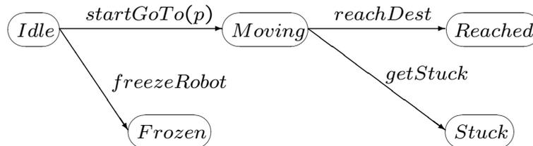
Also action  $resetRobot$  that returns robot to *Idle* state; can be performed in any state. Also fluents  $robotDestination(s)$  and  $robotPlace(s)$ .
