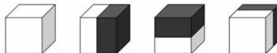
Figure 6: The set of cuboid filters used by Ke et al. (Ke, Sukthankar & Hebert, 2005). Each filter is composed of cuboid volumes, where the white and black volumes within the features are associated with 1 and -1, respectively.
