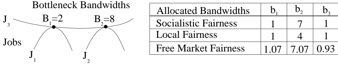
Figure 3: The following example demonstrates Socialistic, Local, and Free Market Fairness. There are two bottlenecks with capacities B_1 = 2 and B_2 = 8 . There are three jobs with J_1 passing through B_1 , J_2 through B_2 and J_3 through both. Socialistic Fairness allocates b_1 = b_3 = 1 bandwidth to jobs J_1 and J_3 , fairly splitting the bandwidth of B_1 = 2 . Job J_2 is given the remaining B_2 bandwidth b_2 = B_2 - b_3 = 8 - 1 = 7 because doing so does not hurt the other jobs. Local Fairness allocation is the same in this example, except that J_2 is only given his fair share of B_2 's bandwidth which is b_2 = \frac{B_2}{n_2} = \frac{8}{2} = 4 . Note that the second bottleneck has B_2 - b_2 - b_3 = 8 - 4 - 1 = 3 bandwidth left unused. AIMDEQUI or Free Market Fairness allocates price f_1 to the bandwidth of the first bottleneck and f_2 to that of the second. The key requirements are that the bottlenecks are at capacity, giving b_1 + b_3 = B_1 = 2 and b_2 + b_3 = B_2 = 8 and that all players pay the same for their bandwidth giving that f_1 \cdot b_1 = f_2 \cdot b_2 = (f_1 + f_2) \cdot b_3 = \frac{\alpha}{(1-\beta)} . Changing this constant, simply scales the prices and hence wlog \frac{\alpha}{(1-\beta)} = 1 . This gives us a total of 2 + 3 = 5 equations and 2 + 3 = 5 unknowns. Solving them gives us that the price for the bandwidths are f_1 = 0.96 and f_2 = 0.14 . Note that as expected the bandwidth through B_1 is much more expensive because there is less of it. J_3 gets b_3 = 0.93 bandwidth, which is less than the others because he is paying more. This leaves b_1 = 1.07 and b_2 = 7.07 for the other jobs.
