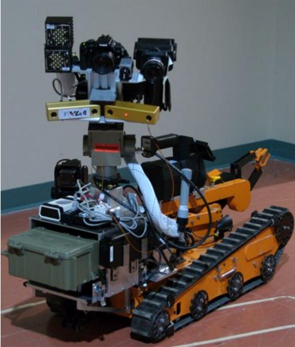
**Figure 2. C2SM sensor mounted on a mobile robot platform. The sensor provides stereo, IR, chemical and radiological modalities.**
