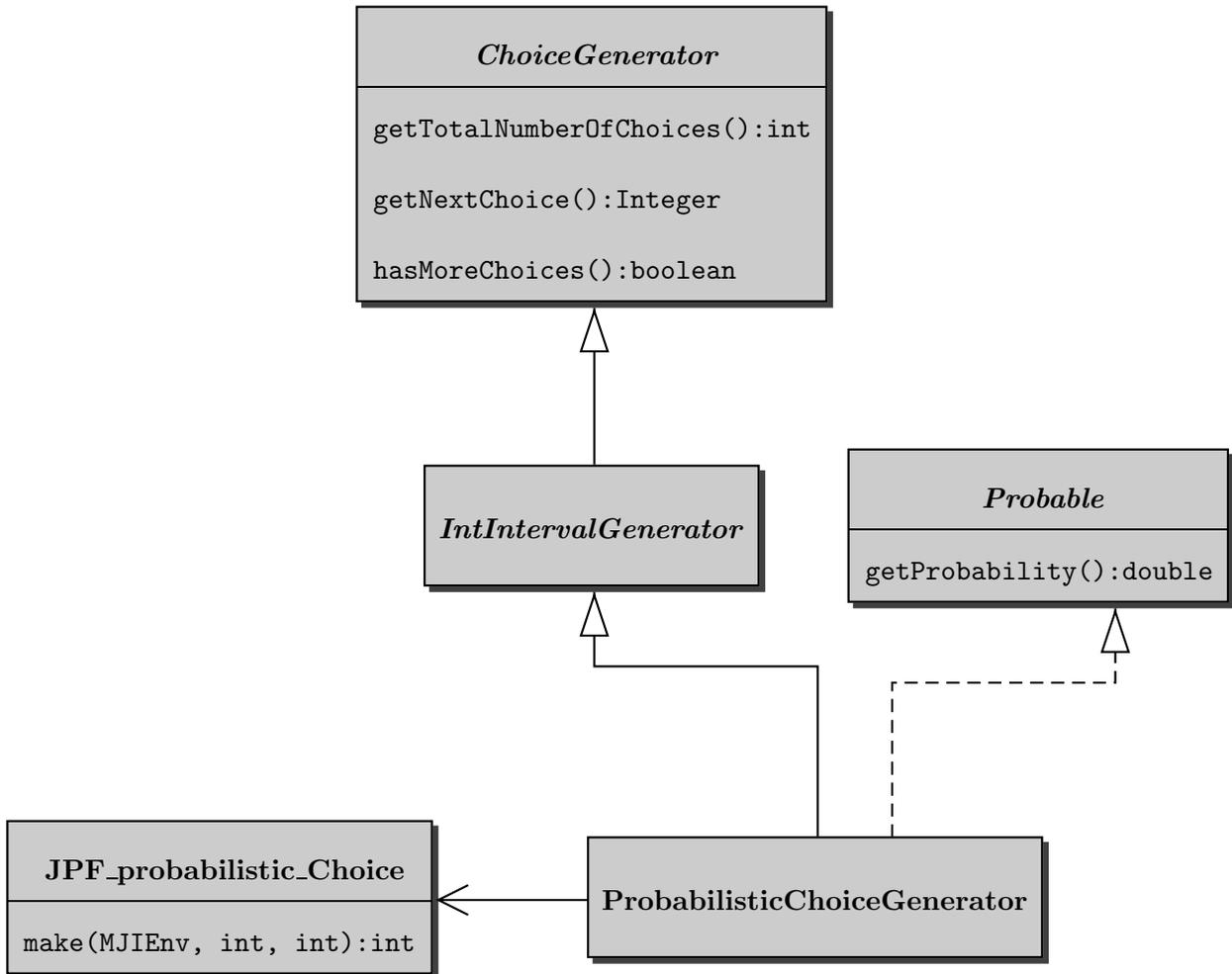
When we are using JPF to model check the following simple example, we can use our classes and interfaces to enumerate the alternatives of a randomized choice.
