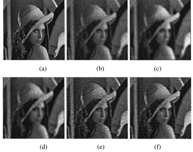
Fig. 3. Image restoration of the Lena image. (a) Original. (b) Noisy and Blurred with out-of-focus blur (MSE = 501.33). (c) Restored image with (3 \times 3) spatial averaging (MSE = 432.24). (d) Restored image with Wiener filter (MSE = 305.13). (e) Restored image with RTS algorithm using causal prediction (MSE = 254.54). (f) Restored image with RTS algorithm using noncausal prediction (MSE = 166.46).
