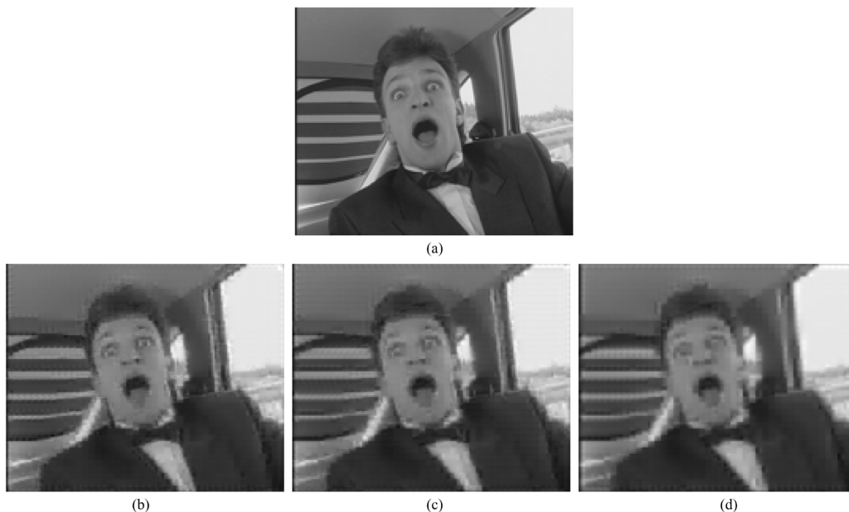
Fig. 9. Comparison of different quality of services. (a) Original frame no. 60 and (b)–(d) frame 60 obtained as part of the video sequence compressed with (b) the Gold service to a bit rate of 125 Kbps ( CR = 48.6 ). (c) the Silver service at a bit rate of 31 Kbps ( CR = 196 ). (d) the Bronze service at a bit rate of 7.75 Kbps ( CR = 784 ). In Silver and Bronze services, gains due to temporal compression are included in the compression ratios.
