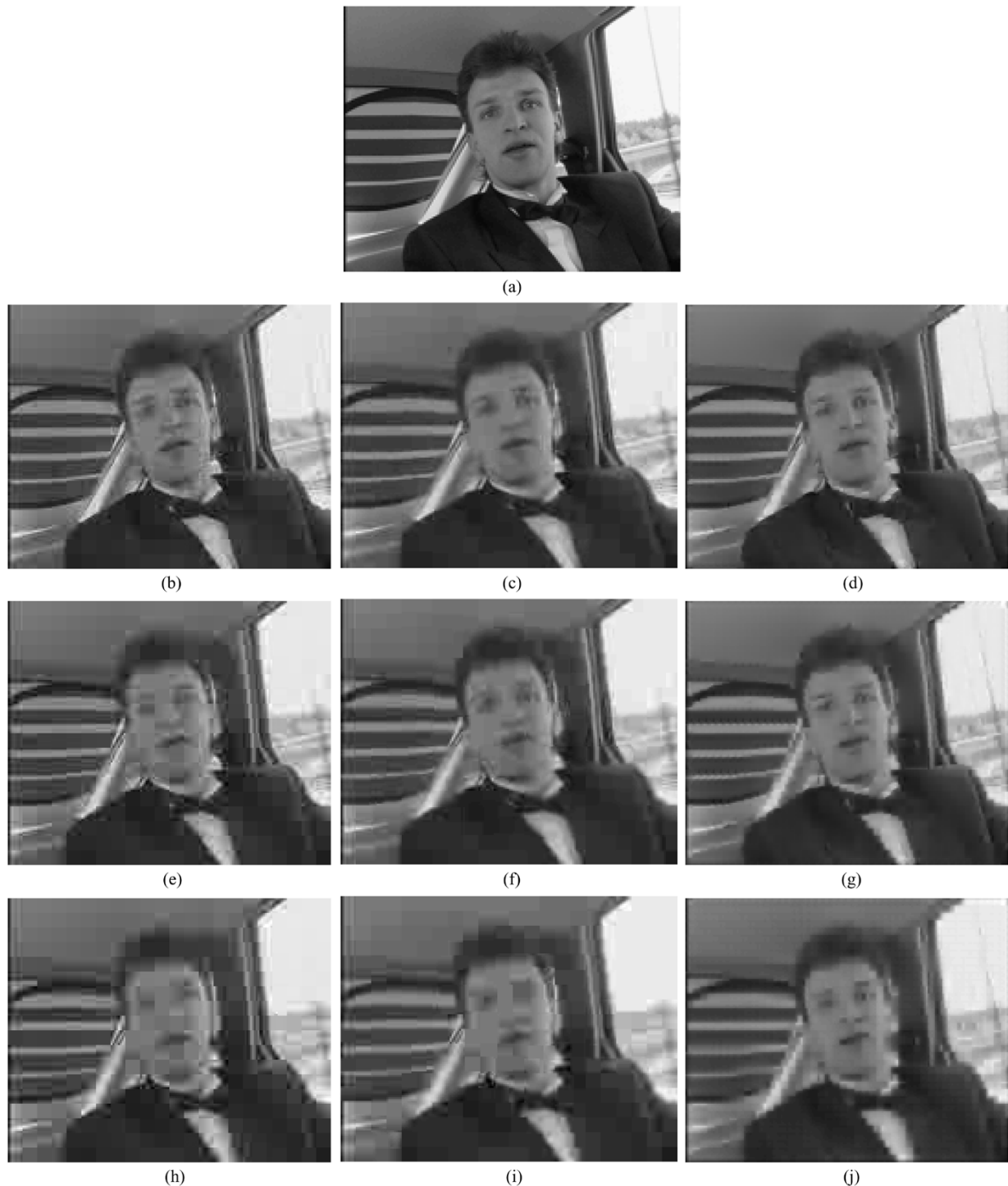
Fig. 7. Frame 21 extracted from the carphone sequence compressed to different bit rates using H.263, MPEG4, and the block SNP/VQR. Frame (a) is the original frame. The frames in the left most column are compressed using H.263, the frames in the middle column are compressed using MPEG4, while the frames in the right most column are compressed using the block SNP/VQR. The bit rate for frames (b), (c), and (d) is 90 Kbps ( CR = 67 ), the bit rate for frames (e), (f), and (g) is 39 Kbps ( CR = 155 ), and the bit rate for frames (h), (i), and (j) is 24 Kbps ( CR = 253 ).
