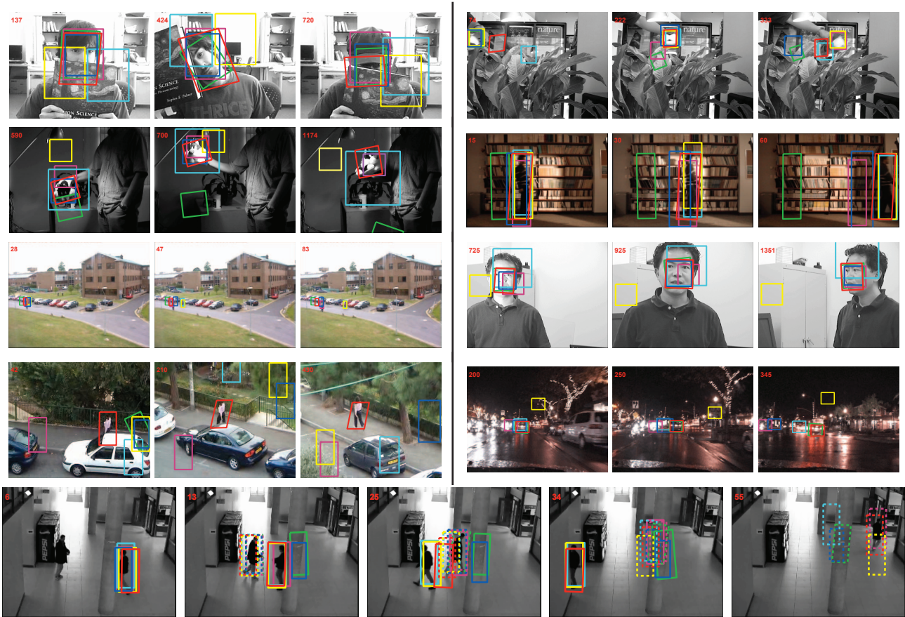
Fig. 3. Qualitative tracking results for the test suite of videos. From top to bottom, left to right, the videos displayed are Occluded Face 2 , Tiger 2 , Sylvester , Illumination , PETS , Ming , Woman , Car11 , and Pop Machines . Red, yellow, cyan, green, purple, and blue boxes correspond to tracking results for PW-SOE, Frag-SOE, MS-SOE, IVT, MIL, and VTD-Int respectively. For the Pop Machines video, two human targets are tracked where the results for the person starting on the right are shown with solid crop boxes and those for the person starting on the left are denoted via dashed boxes.
