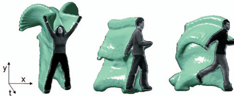
(c) Examples of a spacetime volume (STV) for actors performing a jumping jack , walk , and run actions. Redrawn from [14].
