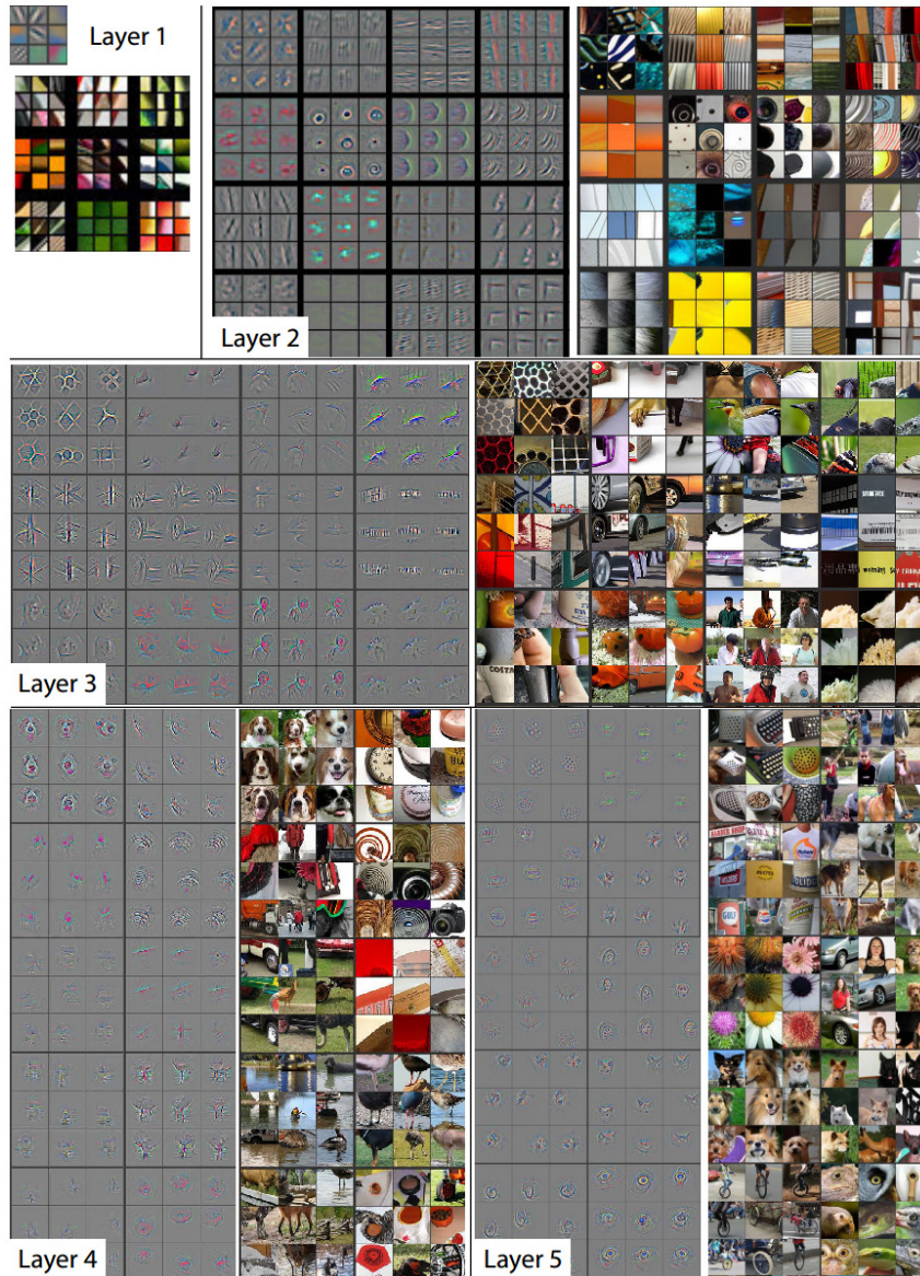
Figure 4.2: Visualization obtained by applying DeconvNet at various layer of a standard ConvNet architecture such as AlexNet [88]. Figure reproduced from [154].
