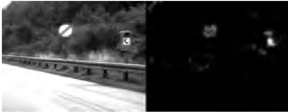
Figure B.4: Left – input image, Right – saliency map. This model reproduces the results presented by Itti et al. (Figure 3 in [Itti et al., 1998]). The model identifies the phone pole as the most salient area of the image, followed by the traffic sign.
