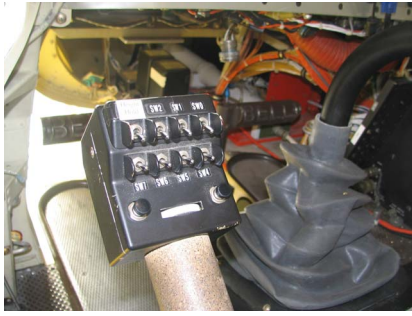
Figure 9. The switches in Bell 412 helicopter which will be used in the detection and discrimination process.
