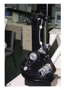
Figure 1. Photograph of the robot used for presenting haptic display to the subject.
