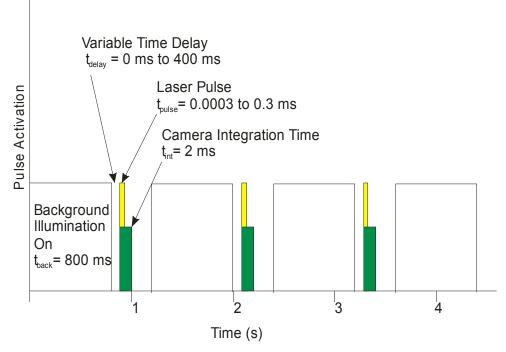
Figure 5 Experimental Control Signals
