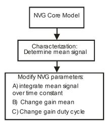
Figure 2 Block Schematic of AGC Model
