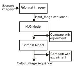
Figure 1 Elements of an NVG Model
