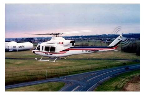
ASRA, can be airborne test facility or fixed base simulator.
