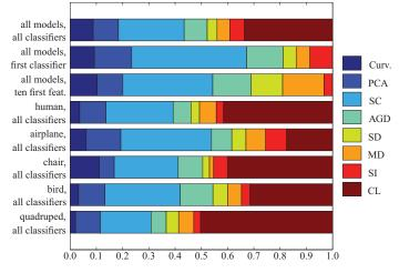
**Figure 5:** Percentages of features used by JointBoost for different cases. See text for details. Legend: Curv.=curvature, PCA=PCA singular values, SC=shape contexts, AGD=average geodesic distances, SD=shape dimeter, MD=distance from medial surface, SI = Spin Images, CL = contextual label features.
