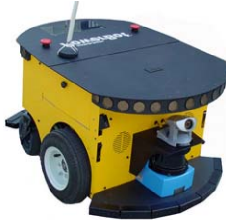
Figure 8. PowerBot™ carries over 100 kg of payload.
