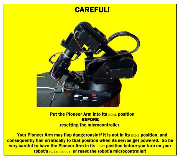
The arm servers also monitor the serial connection with the arm's controller. If the robot's controller does not detect the arm, or if it loses contact with the arm's controller when the arm's servos are enabled, your robot's controller automatically shuts down command and control, and awaits a warm-reset command from the client to re-establish command and control of the Pioneer Arm through the arm servers.
