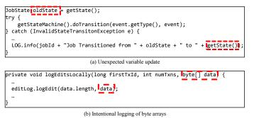
Fig. 7: Code snippets that LCAnalyzer mistakenly flags as logging anti-patterns.
