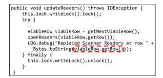
Fig. 1: An example of low quality logging code which caused crash of the HBase server due to a NullPointerException [7].
