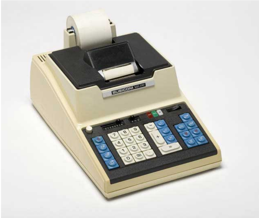
Fig. 16. The Busicom 141-PF – the world's first microprocessor-powered calculator. Source: http://www.4004.com
