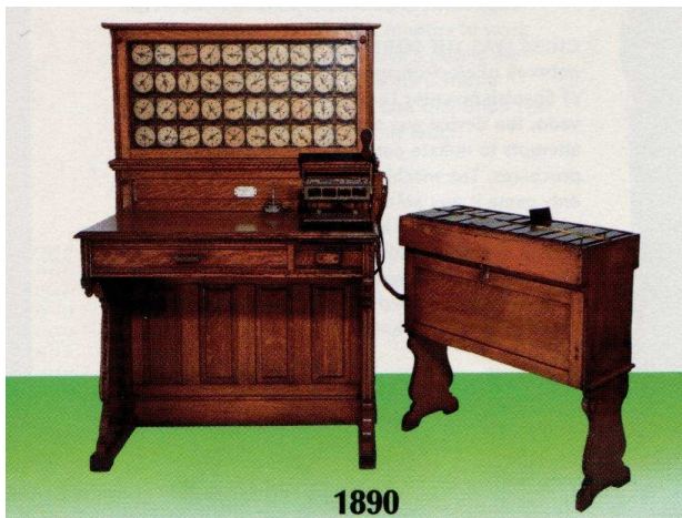
Fig. 3. Herman Hollerith's tabulator (1890). Source: Understanding Computers, Illustrated Chronology and Index , Time-Life Books, 1989
