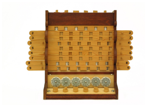
Fig. 15. A replica of a Schickard Calculator. Source: http://archive.computerhistory.org .
