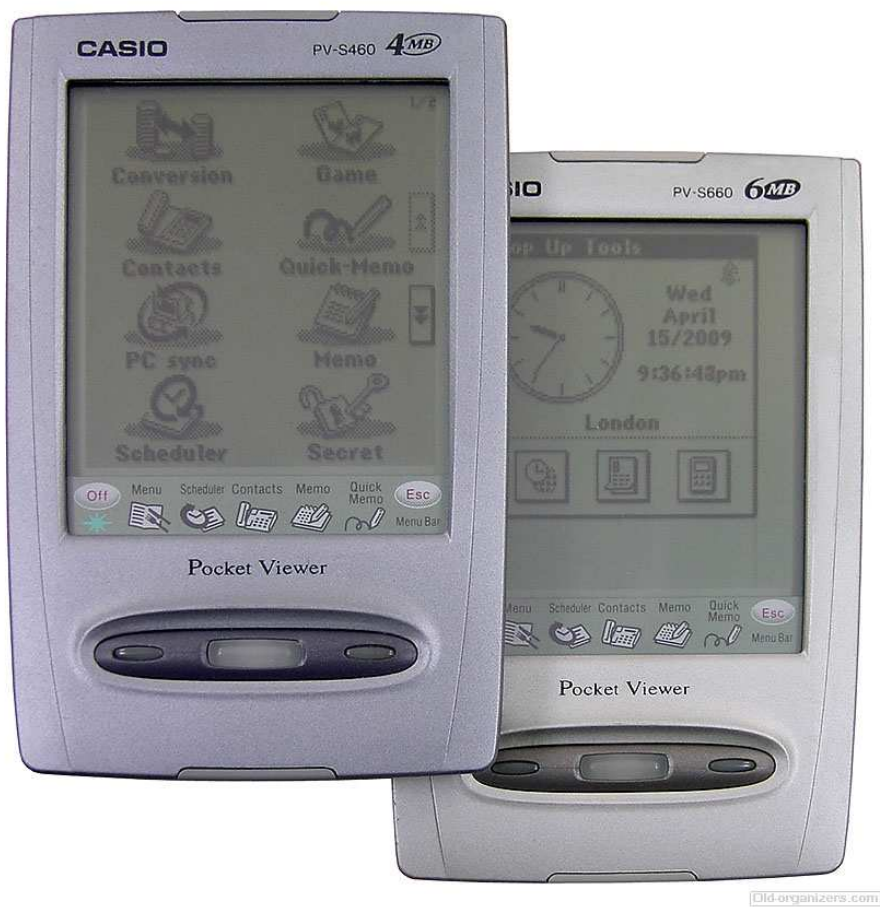
Fig. 25. Casio PV-S460 and PV-S660 pocket viewers, 2000. Functionality: world clock, calculator, currency converter, pocket sheet, expense, contacts, memo, calendar, schedule, to do, reminder alarm, games.
