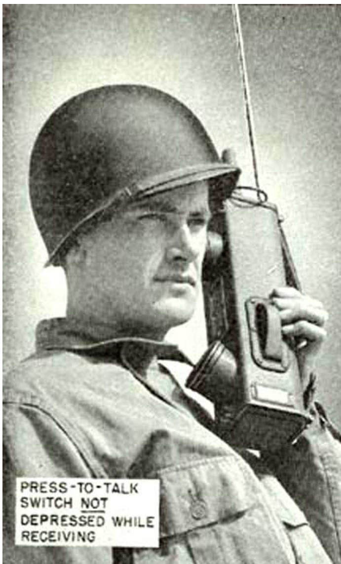
Fig. 5. An early army hand-held "walkie-talkie" SCR536 used by the US Signal Corps during WWII. Source: Motorola M 11-235 manual; scanned by LuckyLouie.
