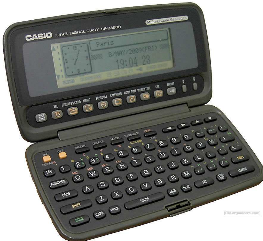
Fig. 23. The Casio Digital Diary SF-8350R, 1994. It offered” phone book business cards, memo, secret memory area, schedule, graphic clock, world time calendar and calculator. Source: http://casio-pda.wikidot.com/sf-8350r
