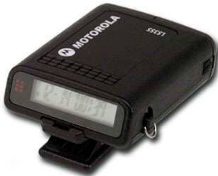
Fig. 11. Motorola pager with a simple one-line display. Source: unknown
