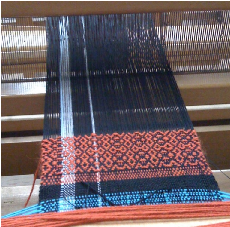
Fig. 9. Weaving is done row by row along the so-called warp threads...
