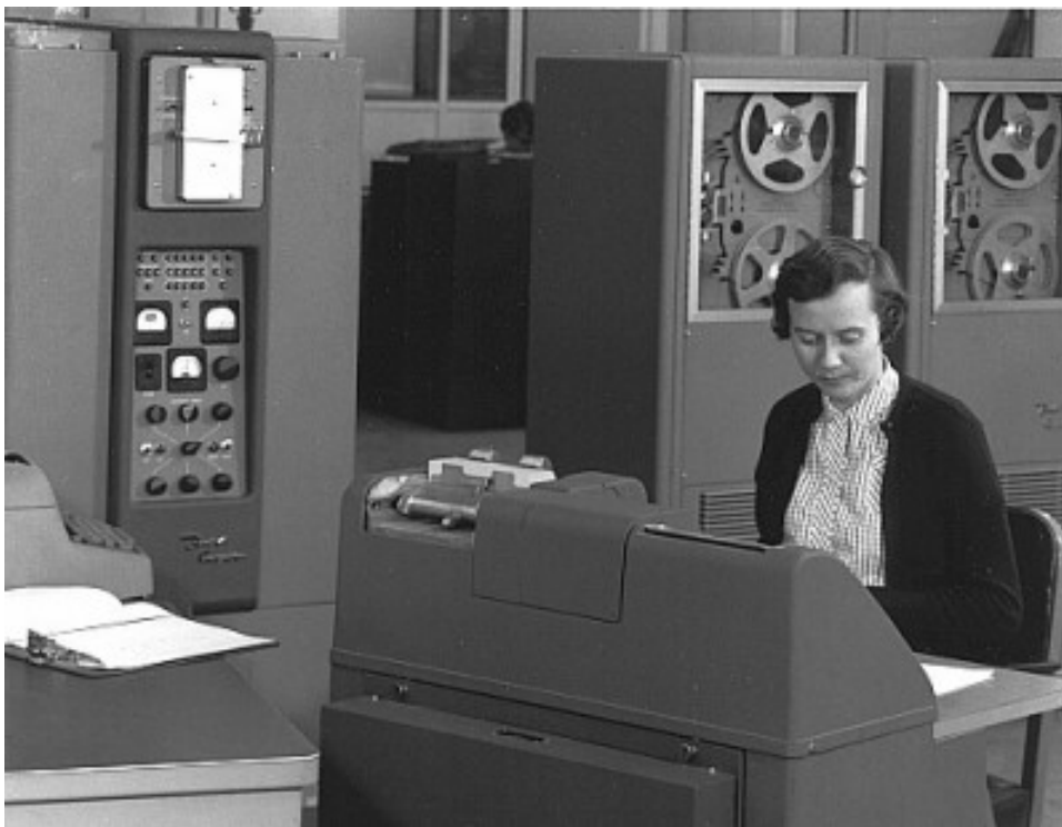
Fig. 17. Magnetic tape equipment attached to a Bendix G-15 computer. Several of such computers were installed at the University of Manitoba. Source: Keith Smillie, http://webdocs.cs.ualberta.ca/~smillie/ComputerAndMe/Part14.html
