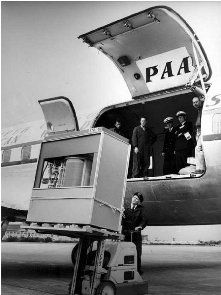
Fig. 18. The first hard drive developed by IBM in 1956 for its Ramac 305 computer had just 5 Mega bytes (Mb) of storage capacity (or 5 million characters). Source: Kyle VanHemert, http://www.gruponeva.es/blog/noticia/7331/el-disco-duro-de-5-mb-lanzado-por-ibm-en-1956-que-pesaba-mas-de-una-tonelada-fotos-retro.html
