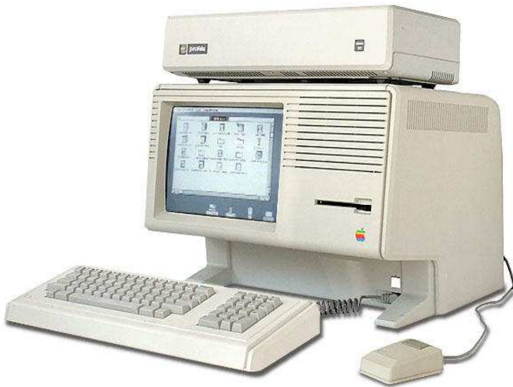
Fig. 13. The Apple Lisa was one of the earliest computers with graphical user interface. Source: oldcomputers.net/lisa.html
