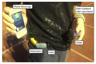
Figure 2. A participant in our study wearing multiple devices. A mechanical clicker was used to record number of steps.
