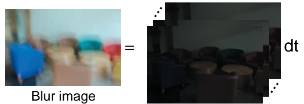
Fig. 3. Our input image is considered the integration of an image scene under projective motion.
