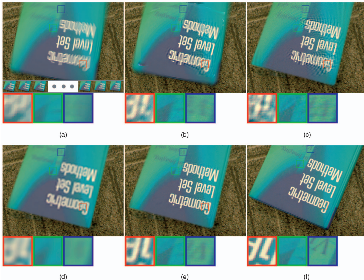
Fig. 12. Image deblurring with spatial varying kernels from rotational motion. (a) Input. (b) Result generated with the method of [42] (obtained courtesy of the authors of [42]). (c) Result generated by Ben-Ezra and Nayar [6] using spatially varying blur kernels estimated from optical flow. (d) Result generated by back projection [21]. (e) Our results. (f) The ground-truth sharp image. Close-ups are also shown.
