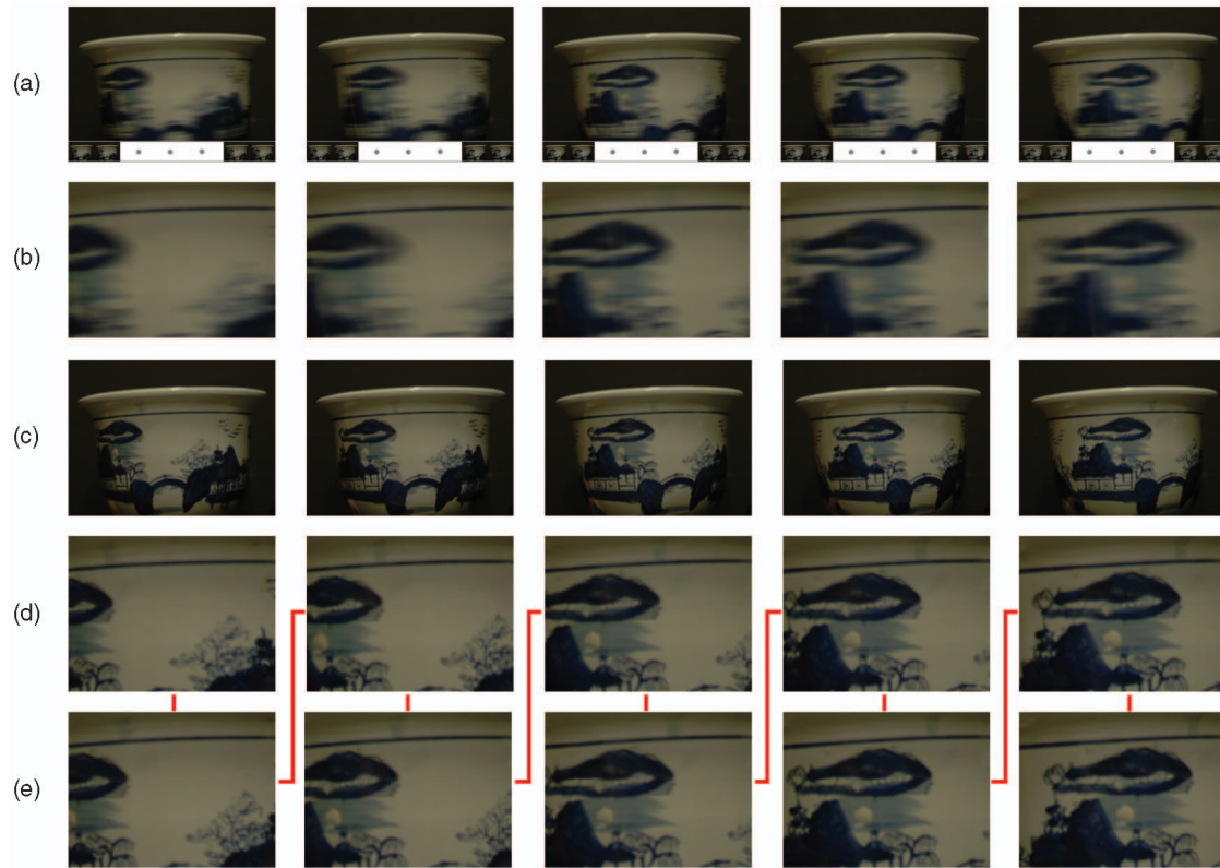
Fig. 17. Video deblurring with out-of-plane rotational motion. The moving object is a vase with a center of rotation approximately aligned with the image center. (a) Input video frames. (b) Close-ups of a motion-blurred region. (c) Deblurred video. (d) Close-ups of deblurred video using the first low-resolution frames as the reference frames. (e) Close-ups of deblurred video frames using the fifth low-resolution frames as the reference frames. The final video sequence has higher temporal sampling than the original high-resolution video and is played with frames ordered according to the red lines.
