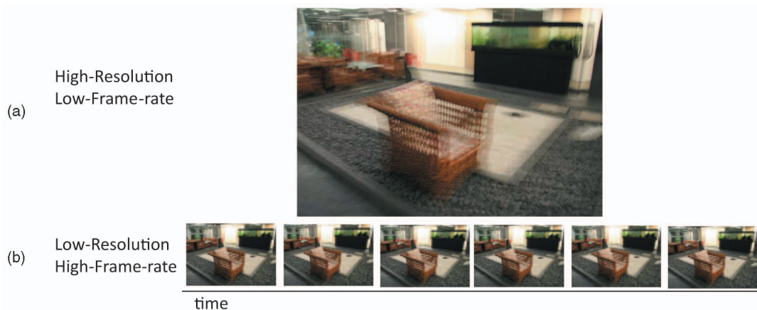
Fig. 1. Trade-off between resolution and frame rates. (a) Image from a high-resolution, low-frame-rate camera. (b) Images from a low-resolution, high-frame-rate camera.
