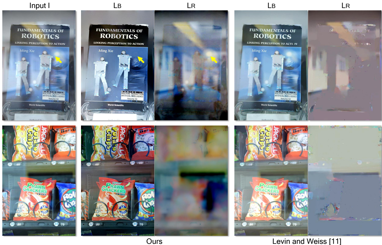
Fig. 7. Two examples of reflection removal results of our method and prior single image approach in [11]. Our method provides visually clearer separation results. But in the top case, a small part of the background is smooth (pointed out by yellow arrow) which breaks our assumption, leading to incorrect separation at that small region (How to correct such cases is shown in Figure 8).
