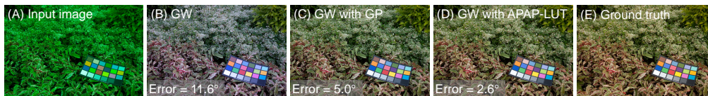
Fig. 4. Projective bias correction of the estimated illuminant of the gray world algorithm (GW) [2]. (A) A raw Canon EOS-1Ds image from the NUS dataset [8]. (B) The corrected image using the GW algorithm. (C) The corrected image using the global projective transformation (GP). (D) The corrected image using the as-projective-as-possible with the lookup table (APAP-LUT). (E) The ground truth image. The images in (B-E) were rendered to sRGB color space for better visualization using the camera-pipeline software of [28].
